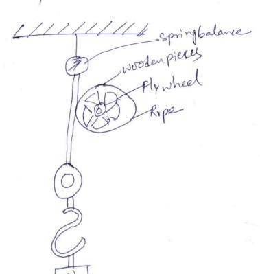
It is another form of Absorption type. It corrists one, two or more ropes wound around the Hyrotheel or oim of a pulley fined rigidly to shaft of an ensure the upper end of ropes kept constant.
