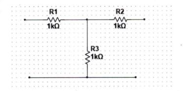
b) Evaluate the ABCD parameters for below circuit
