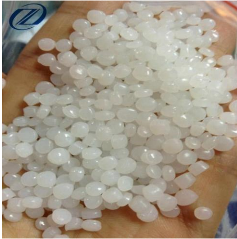
Plastic granules used for blow moulding
